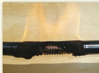
Wardflex 2 (pictured above) does not meet ASTM E84 with respect to flame spread and smoke density.
