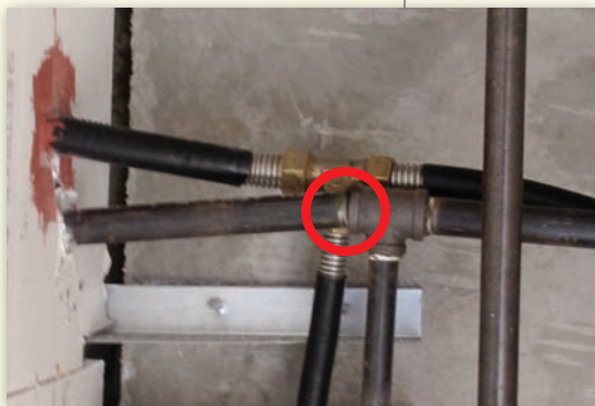
Recent UC San Diego earthquake testing proved that black iron pipe fractured and leaks while the CounterStrike CSST remained leak proof.
