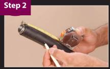
Mark the sleeve at specified length on the Strip Length Chart (above) – plus 2".
