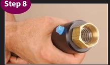
Holding the black coupling, slide fitting up to capture split rings into nut. Be sure split rings slip all the way to the base of the internal threads. Assembly is now ready to be attached to the adapter on the equipment.
