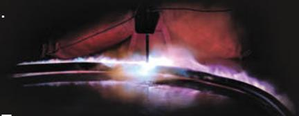
**Simulated lightning test with no product failure**
